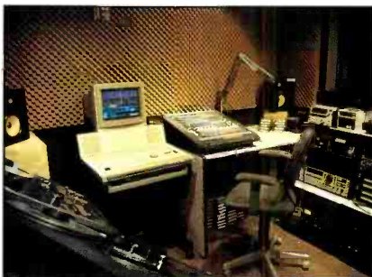
A radio production studio using a virtual multitrack digital production system in an analog-interfaced application.
