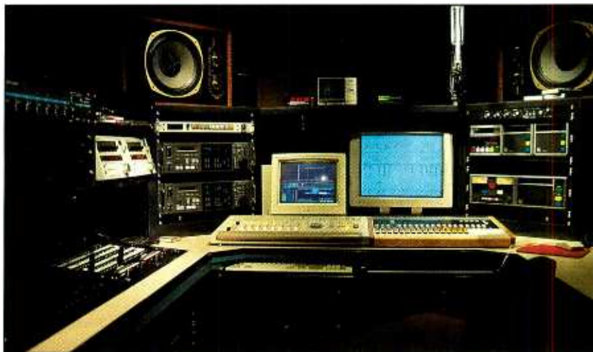
A virtual multitrack digital production system in an all-digital (digitally interfaced) radio control room.
